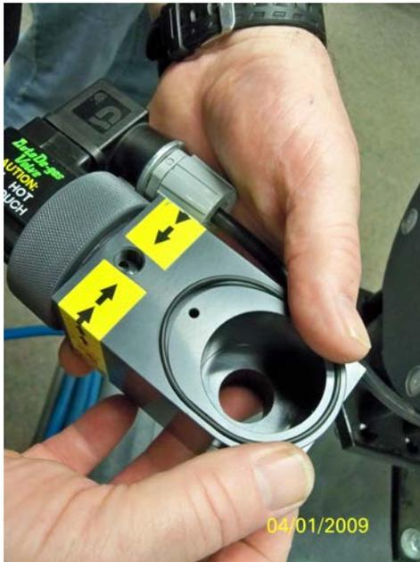
Install the lower O-ring to the valve.
