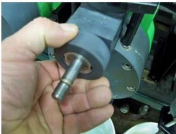
5. Remove Core Tube Assembly.
