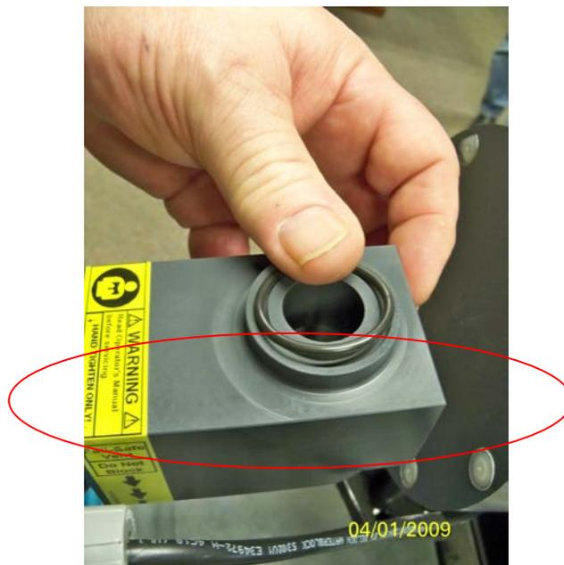
Install the top O-ring to the valve body.
