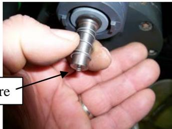
Check that small spring is inserted in Core
