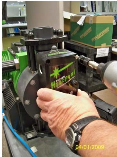
Remove the front cover from the old Hypo valve enclosure.
