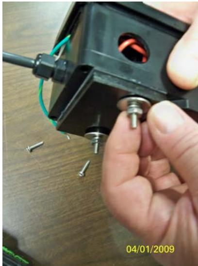
Remove the two nuts, lock washers and flat washers.
