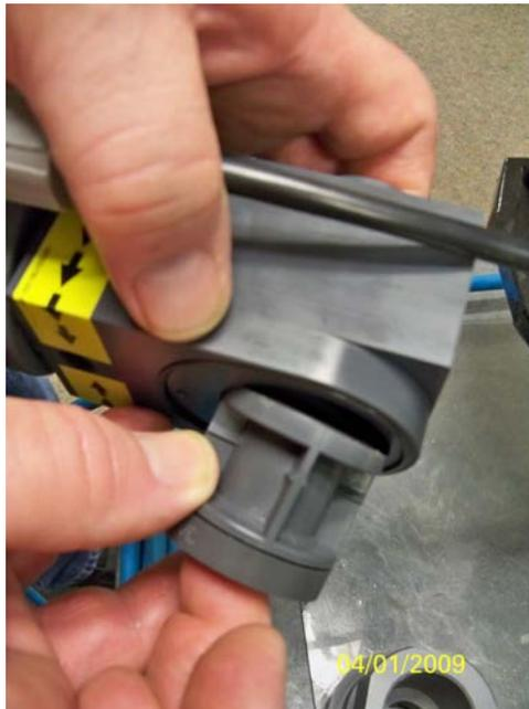
Insert the check valve assembly into the valve body.
