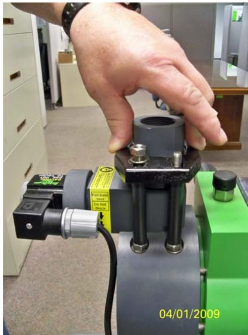
Apply even pressure to the Tie Bar to align the parts and next tighten the tie bar nuts. Tie bar bolts are tightened to 10 in. lb. of torque and additional tightening may be required to stop any leakage.
