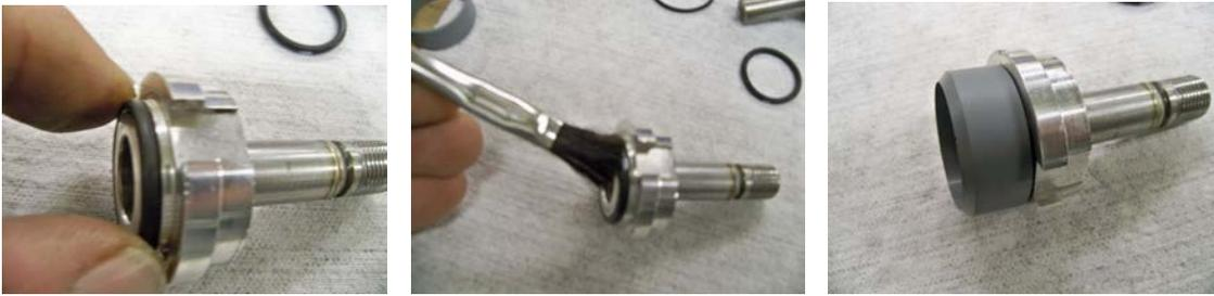
11. Install NEW O-ring on Seal Kit and with lubricant that is compatible with product being pumped.
