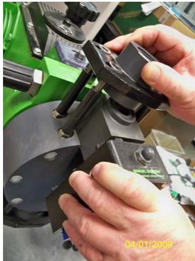
Loosen or remove the tie bar nuts and lift the valve cap to remove the hypo valve assembly.
