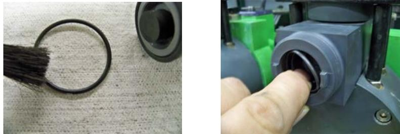
13. Install NEW Seal Kit into Valve Body. Use care to ONLY push straight into bore.
