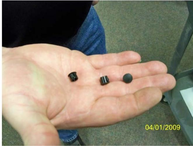
Install the 4 screw dust caps to the front cover of the electrical enclosure.
