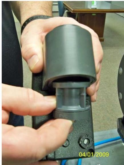
Remove the check valve assembly.
