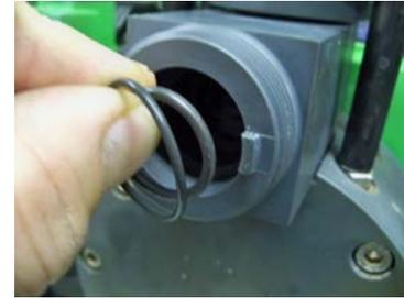
8. Remove the sleeve from the Core Tube and remove the O-ring.
