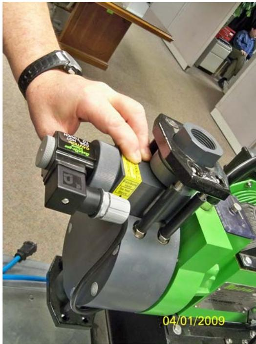
Replace the valve cap and tie bar.
