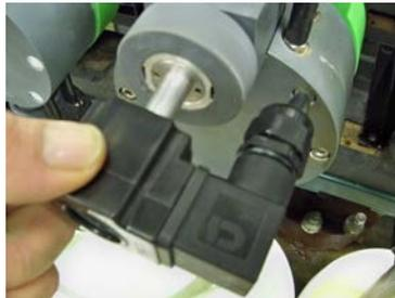
4. Loosen and remove the Union Nut. At this point fluid being pumped may be released from the assembly.
