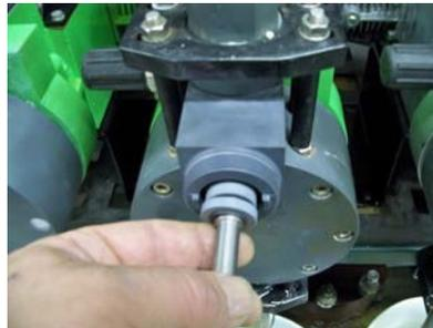
14. Install new spring over Core and check that Small Spring is still in the Core.
