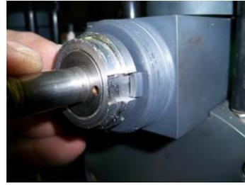
16. Slide Union Nut over Core Tube and tighten onto Body. Do not over tighten, hand tight is sufficient.
