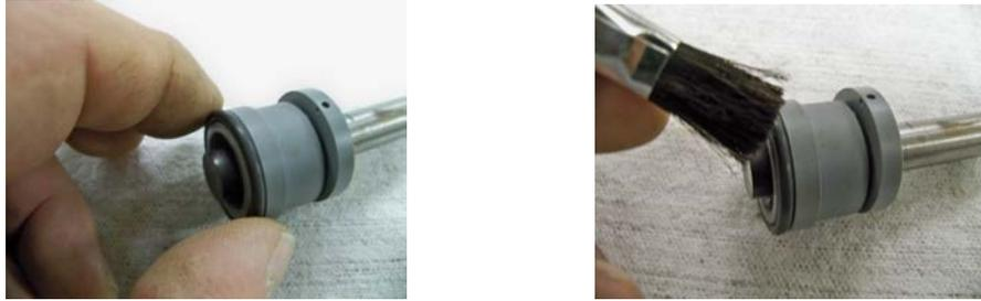
12. Apply a lubricant that is compatible with product being pumped to the Body O-ring and install into Valve Body.
