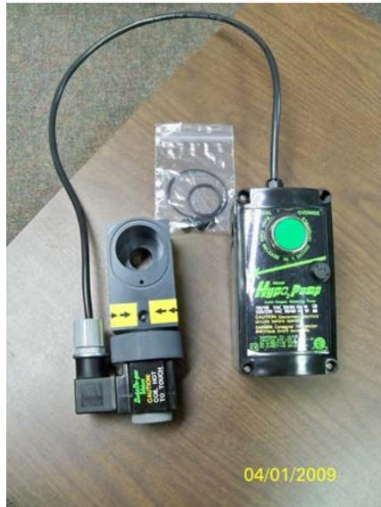
The new Hypo valve comes in three pieces, the valve body assembly with the solenoid, the electrical enclosure and the O-ring package. The solenoid and the electrical enclosure are prewired.
