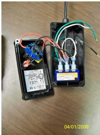
Remove the front cover to expose the wiring and the mounting screws.
