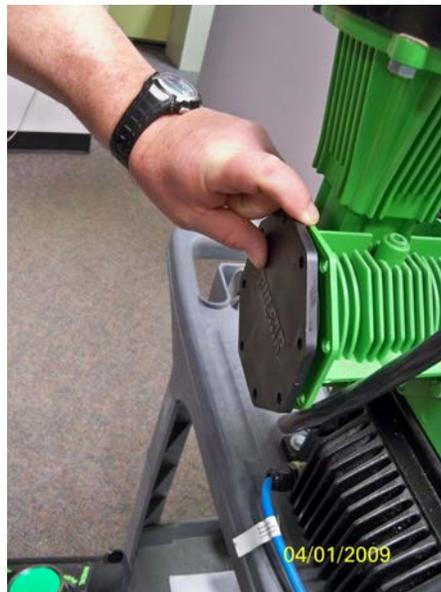
Remove the plastic cover from the end of the gearbox.
