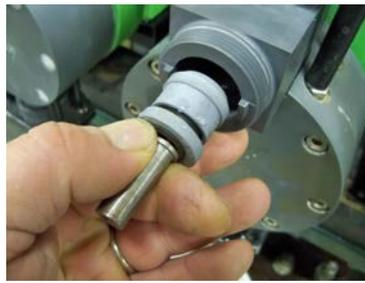
7. Inspect Valve Body for O-rings that may have been left in and remove.
