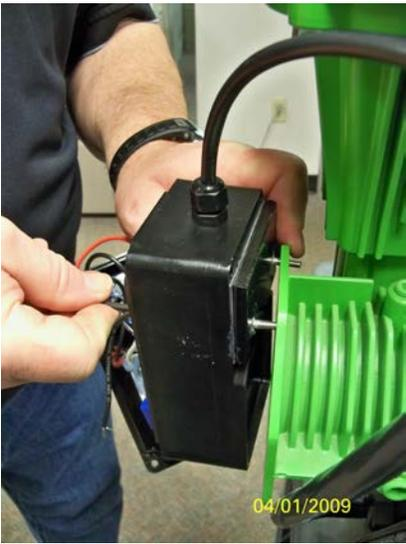
The existing top two holes in the rib of the gear box will line up with the holes in the electrical enclosure. Use a 3.0 mm Allen wrench to tighten the mounting screws, and a 9 mm open end wrench for the nuts.
